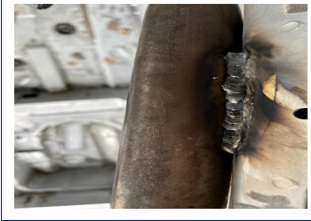
PHOTO 7 FRONT ROLLBAR TO "A" PILLAR ATTACHMENT
