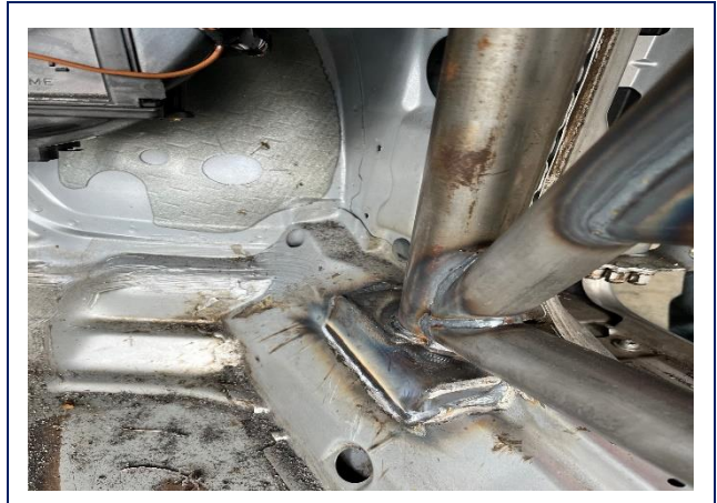
PHOTO 6 FRONT ROLLBAR TO FLOOR ATTACHMENT
